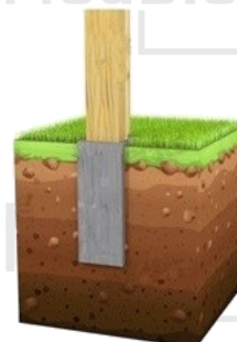
POST CONCRETED IN Onto soft-standing ground
